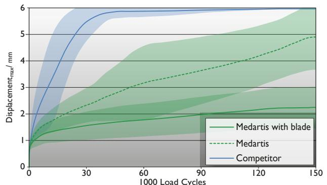
Figure 4: Displacement over time of different proximal humerus plating systems (average and standard deviation)
