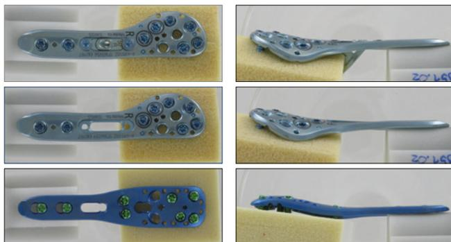
Figure 1: Constructs used for biomechanical testing (from top to bottom: Medartis with spiral blade, Medartis, competitor)
