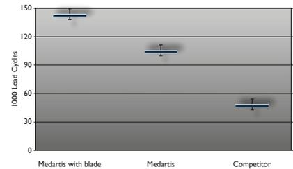
Figure 5: Load Cycles at failure of different Proximal Humerus Plates
