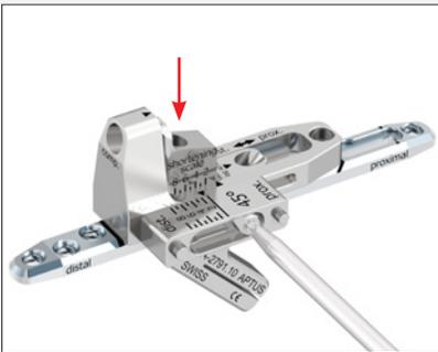
Insert the compression element into the basic element and fix it to the plate using the integrated screw. Tighten the screw with the screwdriver.
